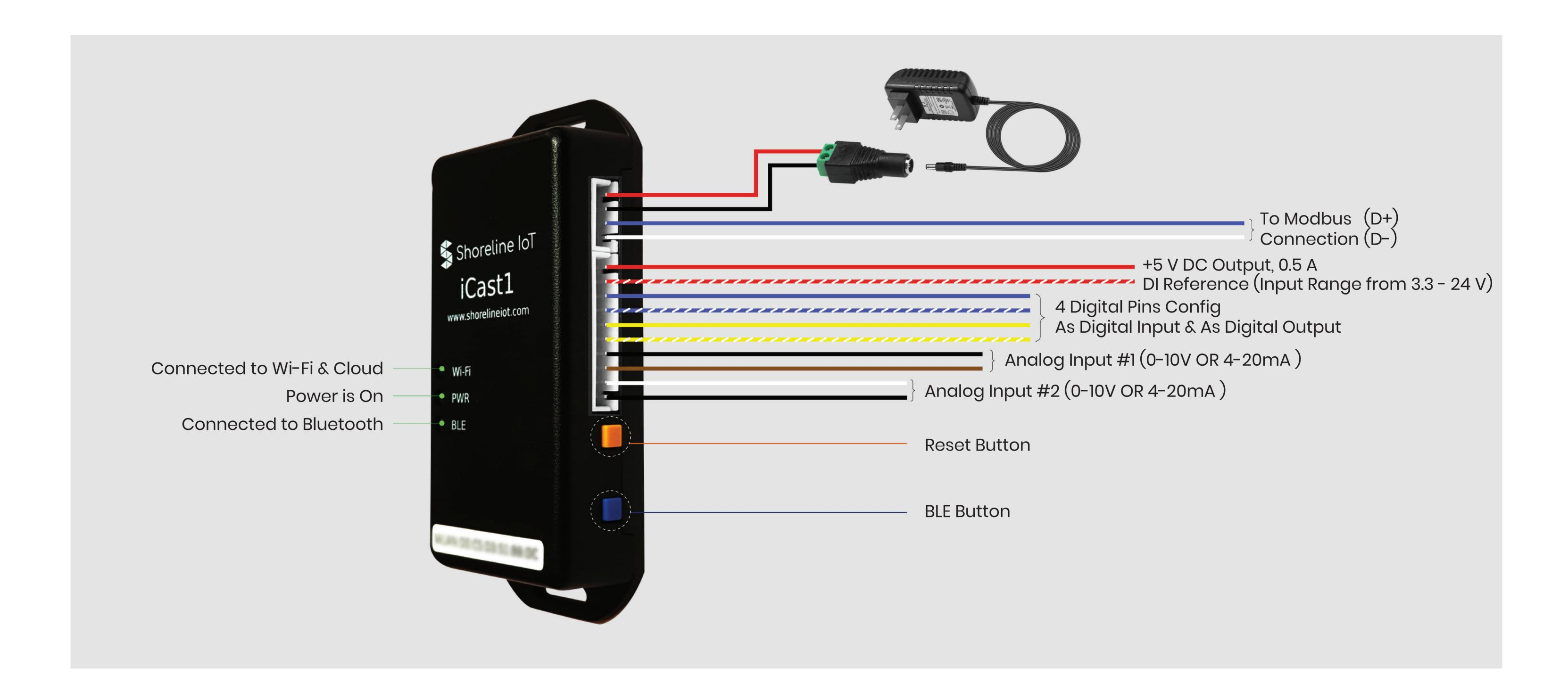
Device Power: Connect 12V power adapter from the package to female DC plug using the 4-pin cable assembly (Red -Positive, Black - Negative)
